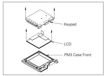
5. Remove rubber keypad and LCD from the PM3 case front.
