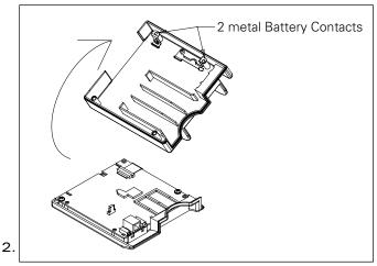
Remove case back. Note the position of the two metal battery contacts.
