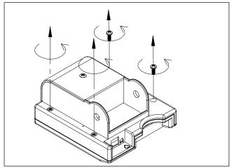
Unplug all wires and remove the PM3 from the indoor rower. Loosen the four PM3 case screws. Do not remove the two left screws
