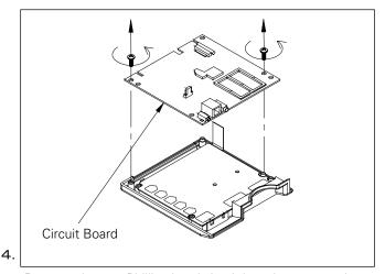
Remove the two Phillips head circuit board screws and remove the circuit board.
